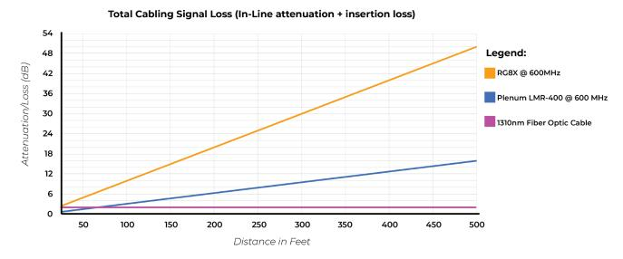
Radio Frequency over Fiberoptic (RFoF) is a straightforward proven solution for the propagation attenuation through coax cables.
